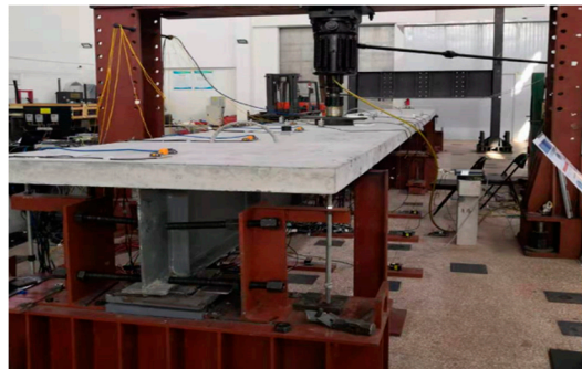
Figure 3. Verified by fatigue tests on bridge model.
