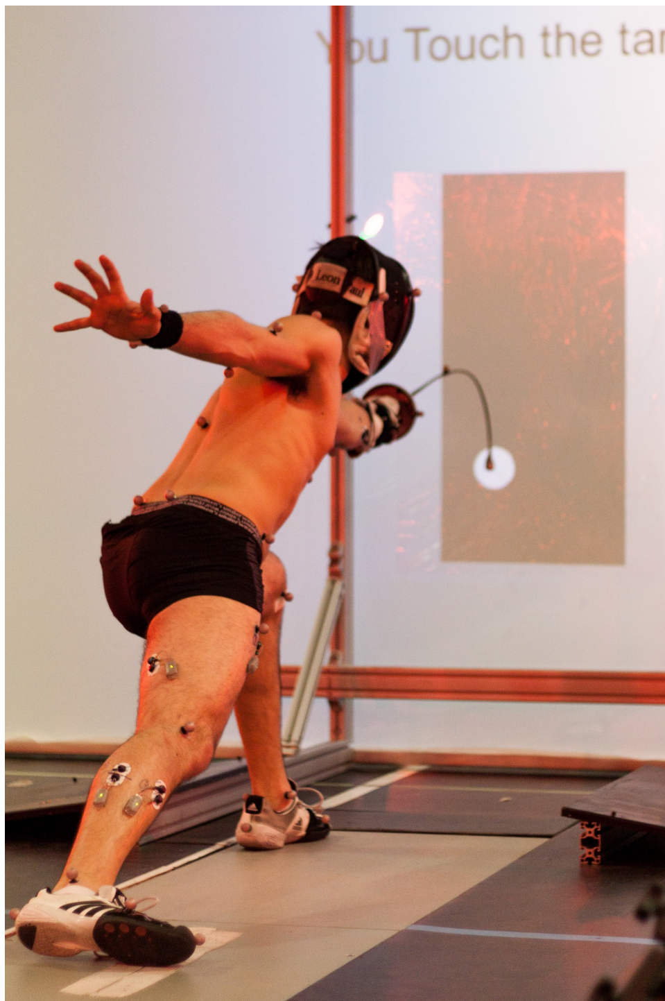
Fig 4. End of a successful lunge trial with a big target (0.10m diameter). Success information was displayed in real time by the system on the top of the plastron. Muscle activity and motion of the fencer were captured for further investigations.
