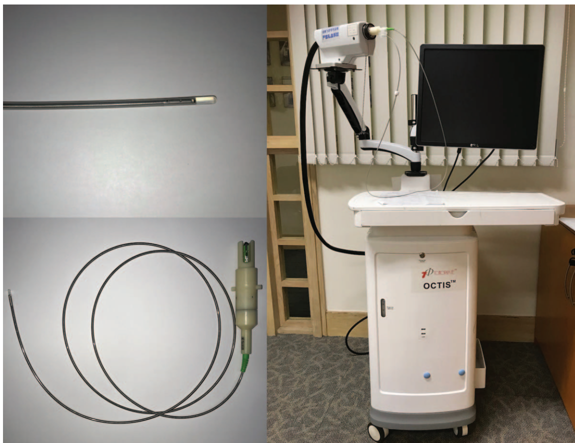
Figure 1. OCTIS with an imaging computing system and a sterile detachable probe. OCTIS = optical coherence tomography imaging system.
