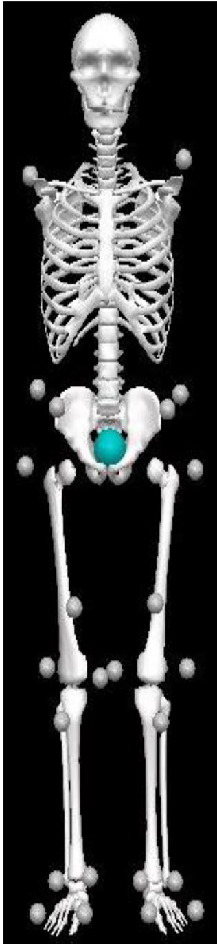
Fig 4. Visual representation of external reflective markers for biomechanical camera tracking. Markers were placed at the sacrum and bilateral shoulders, anterior superior iliac spine, greater trochanter, anterior thigh, medial and lateral epicondyles of the knee, tibial tuberosity, medial and lateral malleoli, heel and medial and lateral forefoot.
