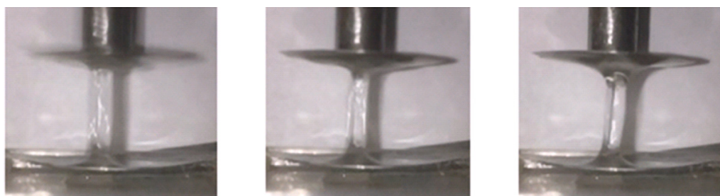
Figure 27. Formation of liquid hydrogel filament (filament lifetime ~0.45 s).
