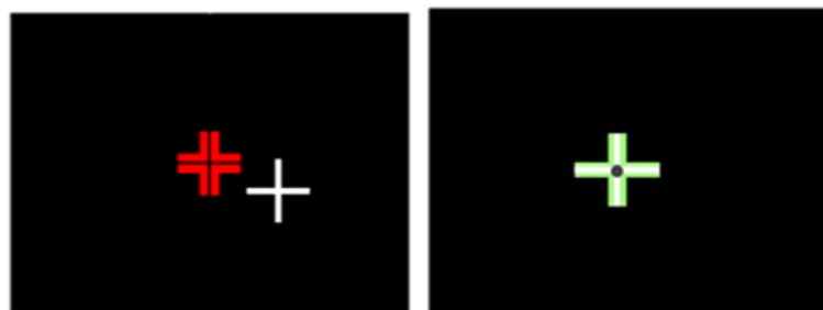
Fig. 2 Visual X-Y direction head positioning and eye fixation feedback. Left image: Patient view requiring moving head laterally. Right image: Patient view when lateral alignment achieved
