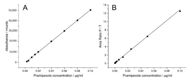
**Figure 5.** Calibration curve of LCW-UV detection system (**A**) of pramipexole (2.5–100 ng/mL) and calibration curve of MS analysis (**B**), where the ratio of the areas of pramipexole and talipexole (area ratio P/T) were plotted against the concentration of pramipexole (0.19–100 ng/mL).
