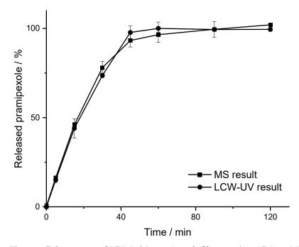
**Figure 6.** Release curve of 0.5% (w/w) pramipexole filaments ( $\overline{m}$  = 17.61 mg) determined by MS and LCW-UV measurement (n = 3,  $\overline{x} \pm SD$ ).
