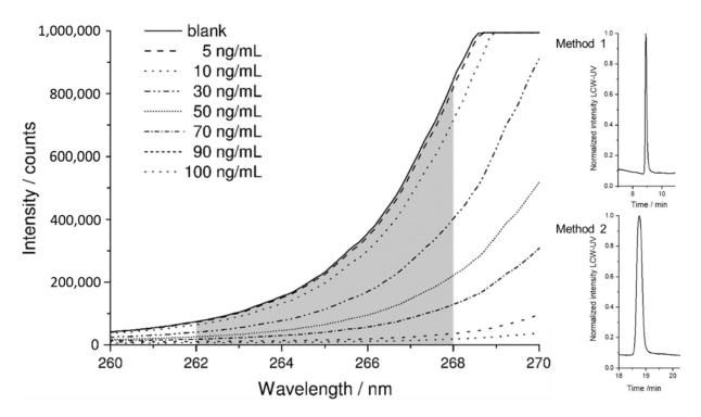
**Figure 4.** Measured intensity of a blank sample and of the peaks of various concentrations of pramipexole (5–100 ng/mL) with highlighted integration range between 262 and 268 nm (grey). Resulting pramipexole peaks (100 ng/mL) after integration for methods 1 and 2.
