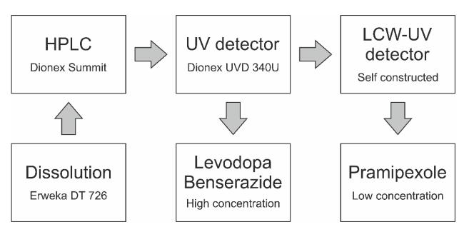
**Figure 2.** Inline coupling of a UV detector and LCW-UV detector for the simultaneous analysis of pramipexole, levodopa and benserazide.
