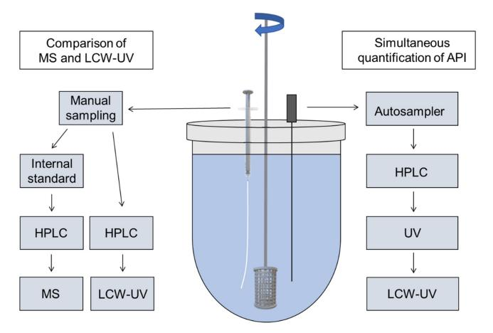
**Figure 1.** Modified dissolution testing with 3D printed basket based on Ph. Eur. monographs 2.9.3 and 5.17.1 with manual sampling (**left side**) for MS and LCW measurement of single pramipexole filaments and automatic sampling (**right side**) for the simultaneous content determination of three APIs (pramipexole, benserazide and levodopa) during dissolution by HPLC-UV and LCW-UV.
