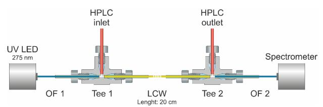
**Figure 3.** Assembly of the implemented liquid-core waveguide ultraviolet detection system consisting of a UV LED (absorption maximum: 275 nm), two optical fibers (OFs 1 and 2), a 20 cm liquid-core waveguide (LCW), two tee pieces and a charge-coupled device detector.
