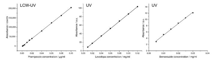
**Figure 8.** Calibration curve of pramipexole measured with the help of the LCW-UV detection system (1–100 ng/mL); calibration curves of benserazide (5–30  $\mu$ g/mL), and levodopa (10–1200  $\mu$ g/mL) both examined by UV detection.
