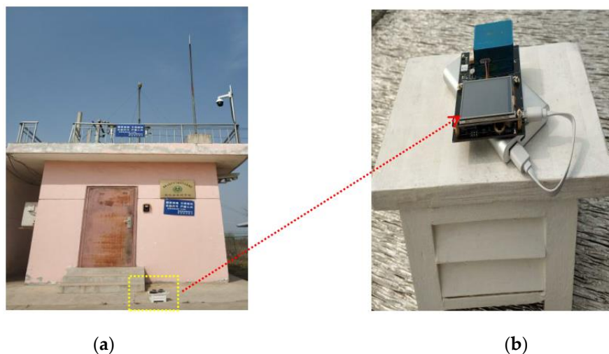
Figure 7. (a) Onborne subsystem calibration test at national air-quality monitoring station; (b) Onborne PM observation subsystem.
