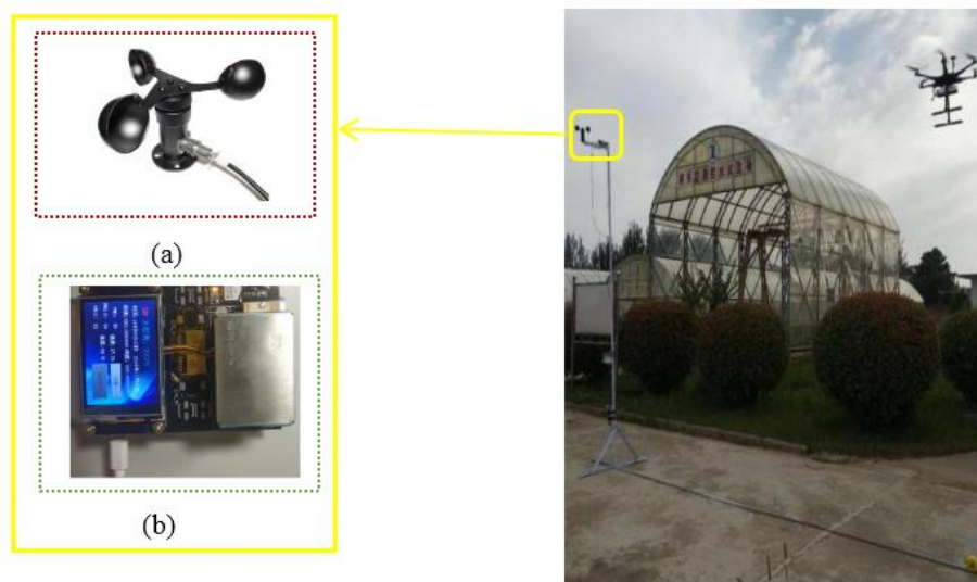
Figure 12. Comparison experiment of fixed tower PM monitoring system and hovering UAV systems. (a) Three-cup anemometer. (b) Fixed tower data collection unit is an onborne PM observation subsystem.
