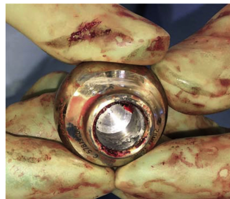
Figure 5. Metal head with fretting corrosion seen within the bore.
