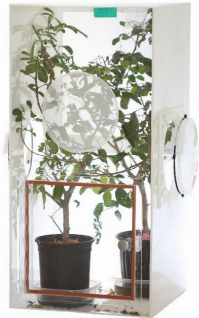
Figure 3. Acrylic box (81.5 × 39.5 × 39.5 cm) used to house two 3.8 L Brazilian peppertree saplings. Access was via a hinged door at the bottom of the front panel, and the back and 20 cm diameter opening on the front were covered in a 250 µm screen for ventilation. The 20 cm diameter side openings were covered in plastic.
