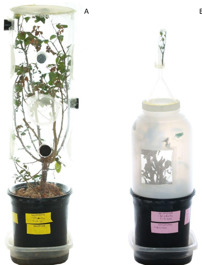
Figure 2. (A) Vented acrylic cylinder placed over a 3.8 L Brazilian peppertree sapling. The cylinder was 45 cm tall and 15.5 cm in diameter. The open top and six 7 cm diameter ventilation holes were covered in a 250 \mu m screen. Rubber stoppers were used to seal 2.5 cm diameter access holes; (B) passive collection apparatus for harvesting newly emerged adult thrips from acrylic cylinder cages. Adult thrips walked up the 3.8 L opaque jar into an inverted funnel and then accumulated in a small tube into which the spout of the funnel was inserted. The tube contained a leafy cutting of fresh Brazilian peppertree for food.
