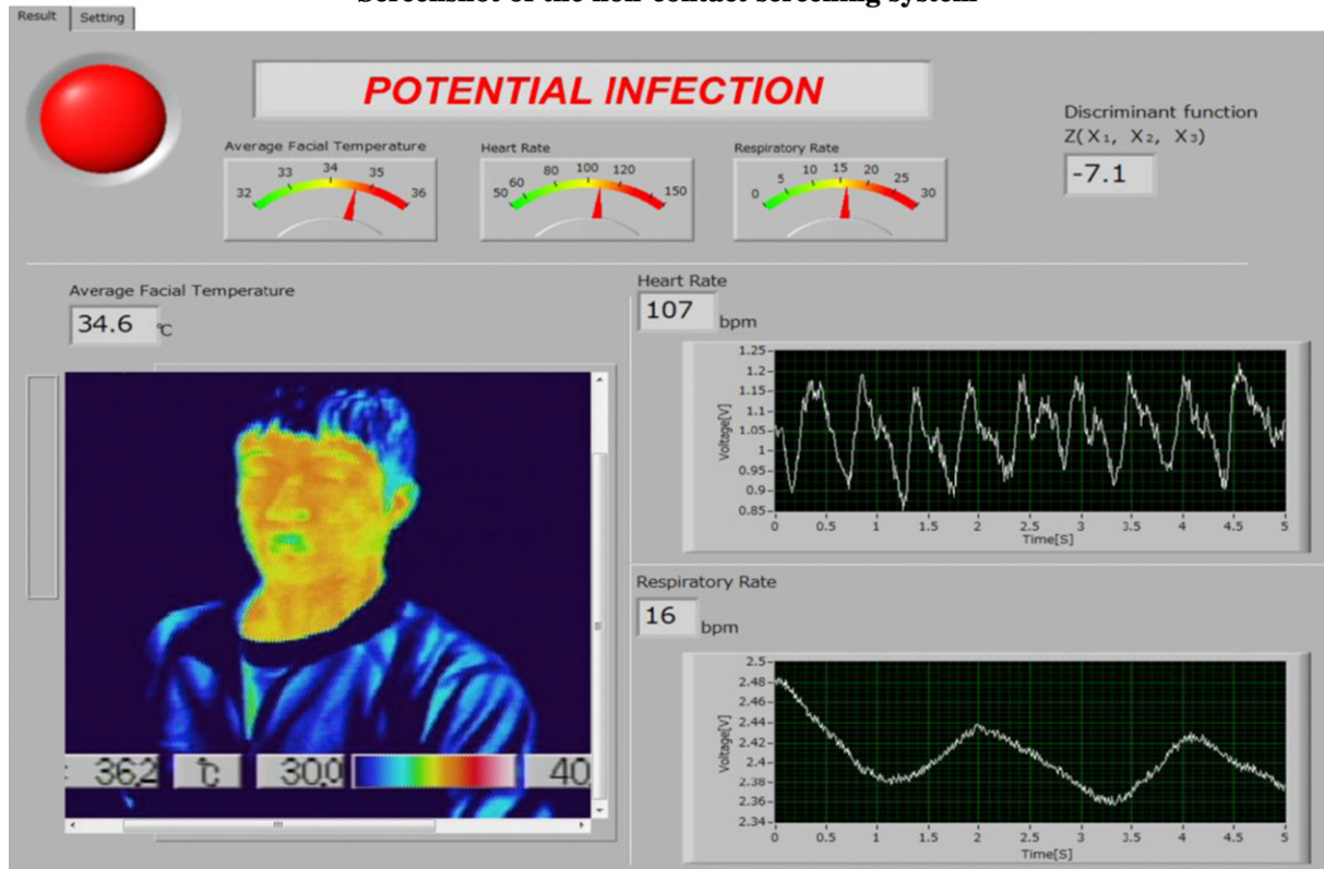
Figure 6 Screenshot of an individual being analyzed using the non-contact screening system. The heart and respiratory curves, the facial temperature mapping, and the screening result, i.e., “potential infection” or “pass”, are displayed.
