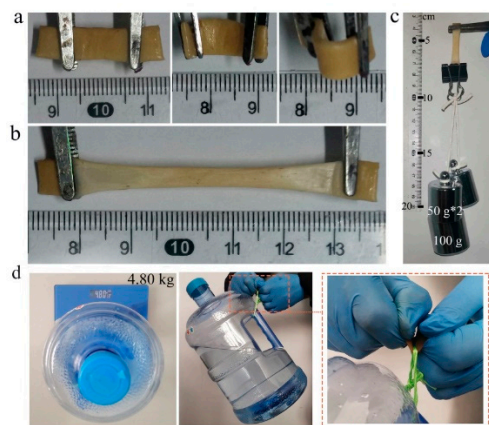
Figure 4. Images of 20.0 wt% PVA–TA24 gel mechanical properties: (a) bending, (b) stretching, and (c,d) holding a weight of 200 g and 4.80 kg.
