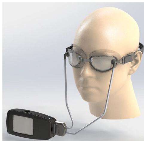
Figure 1. The multi-pressure dial, which includes the goggles connected to a pressure-modulating pump.
