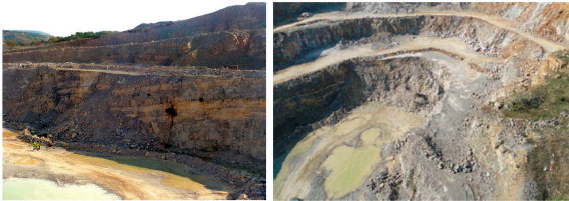
Figure 2. Exposed Middle Triassic carbonates in the operating quarry (left: view from NE, right: image captured from the UAV).
