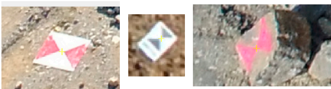
Figure 4. Three types of the GCPs, images taken from the UAV.
