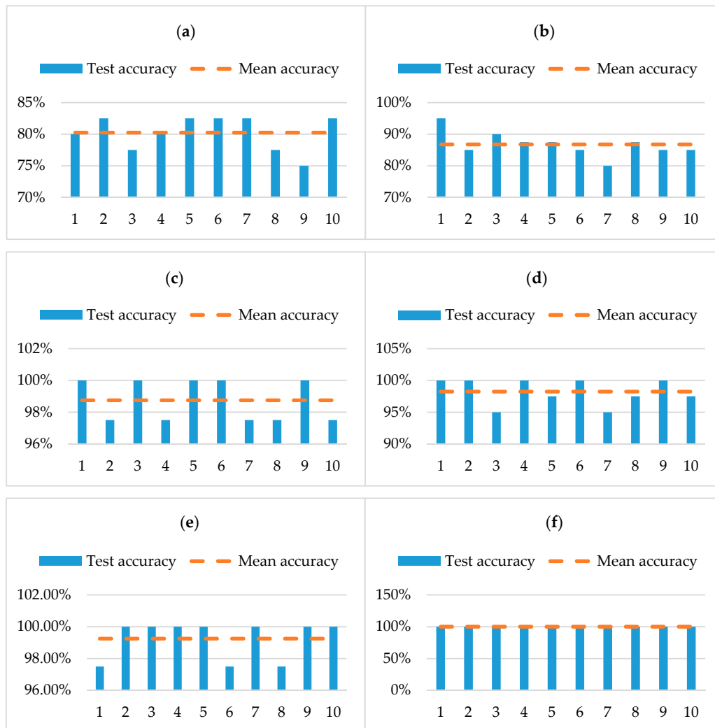
Figure 18. Classification results of fault identification with different characteristics of case 1. (a) Classification result of the original fault signals and sample entropy (SE-OFS), (b) classification result of the SE-EMD, (c) classification result of the SE-EEMD, (d) classification result of the MSE-OFS, (e) classification result of the MSE-EMD, (f) Classification result of the MSE-EEMD-WSST.
