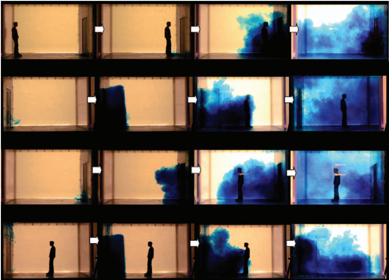
Figure 6. Double-hinged door snapshots (sideviews only; left-to-right). The series of 4 snapshots with each door-opening, manikin movement scenario were taken with respect to the following events, rather than at specific times: food dye movement due to door-opening motions alone then with any initial manikin movement – manikin interaction and any entrainment food dye – final food dye movements once the manikin had come to rest at its destination position. All movement parameters are shown in Table 2 for these double-hinged door ‘fast’ scenarios. A. Manikin moving into the isolation room (seen from outside, V_1 = 0.71 in water (1.1 in air) m/s, angular velocity = 163.1 in water (25.3 in air) deg/s.). B. Manikin moving into the isolation room (seen from inside), V_2 = 0.88 in water (1.36 in air) m/s, angular velocity = 163.1 in water (25.3 in air) deg/s. C. Manikin moving out of the isolation room (seen from outside), V = 0.73 in water (1.14 in air) m/s; angular velocity = 163.1 in water (25.3 in air) deg/s. D. Manikin moving out of the isolation room (seen from inside), V = 0.73 in water (1.14 in air) m/s; angular velocity = 163.1 in water (25.3 in air) deg/s. doi:10.1371/journal.pone.0066663.g006
