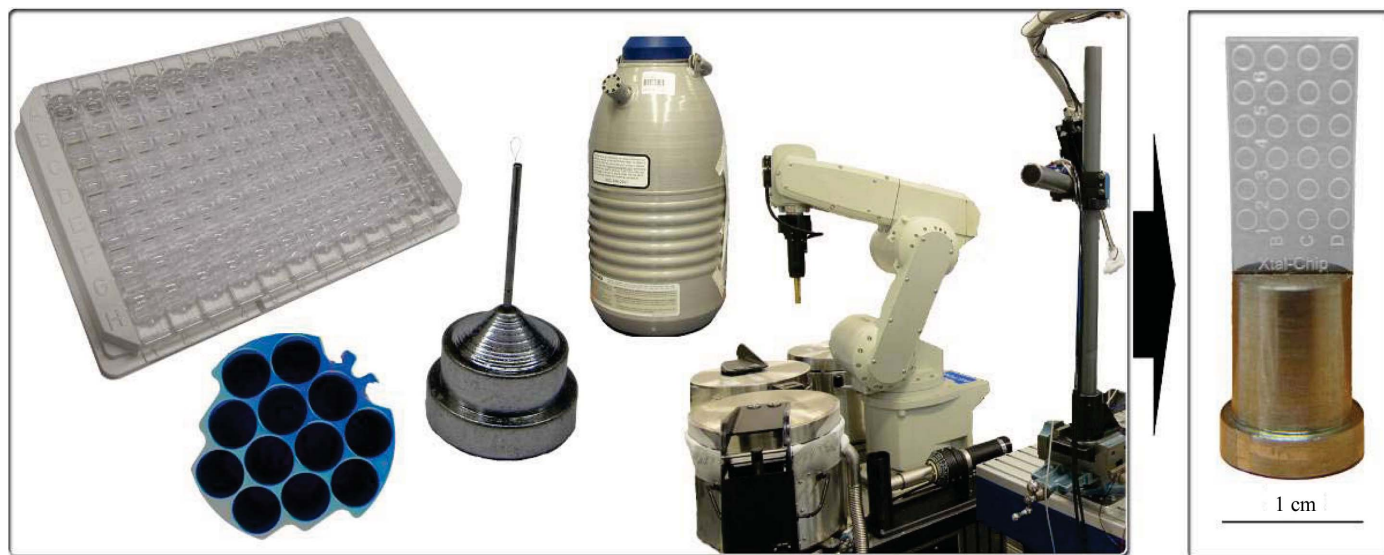
Figure 1 The X-CHIP was designed and developed as an alternative to the conventional stages of the existing crystallization to data collection process.
