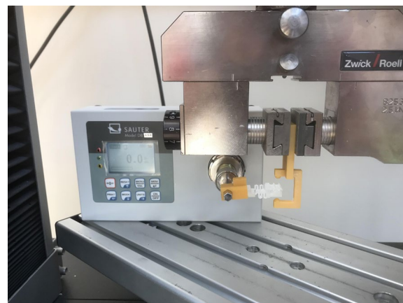
Fig. 4 Testing process (Seen above, the C shaped construct and the reference key locking a spring in place for testing with the Z010 Zwick/Roell (Ulm, Germany) upon initiation the C shaped will be shifted up and down so that each end delivers forces onto the spring which are then recorded by torque device (Sauter DB 0.5-4, Grindelwald, Switzerland) this process is repeated five times total in both directions for every spring tested)
