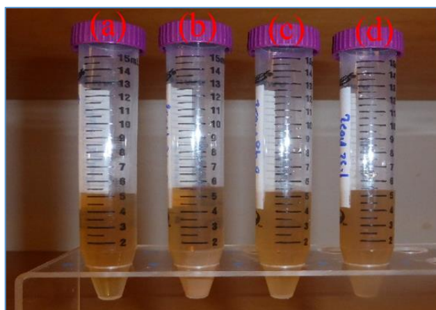
Figure 14. Drilling fluids (Filtrate loss): (a) Ref (5.2 mL), (b) Ref + 0.09 wt.% (5.5 mL) (c) Ref + 0.19 wt.% (5.4 mL) (d) Ref + 0.26 wt.% (5.4 mL).
