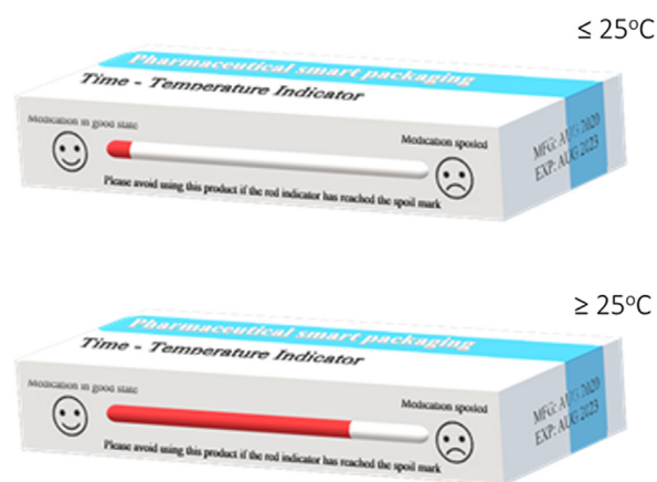
Fig. 5. Illustrating an example of how Time-Temperature Indicators may be utilised as a solution to warn consumers when medication has been exposed to conditions outside those specified by the manufacturer. The horizontal bar undergoes a change in color from white to red (starting from the left side) when RT is greater than a specified limit. The rate of change can be made proportional to RT, where no change takes place if RT is below a specified limit. When the bar undergoes complete change, thus red marker has reached the right side, consumers are advised not to use the product despite remaining shelf-life.
