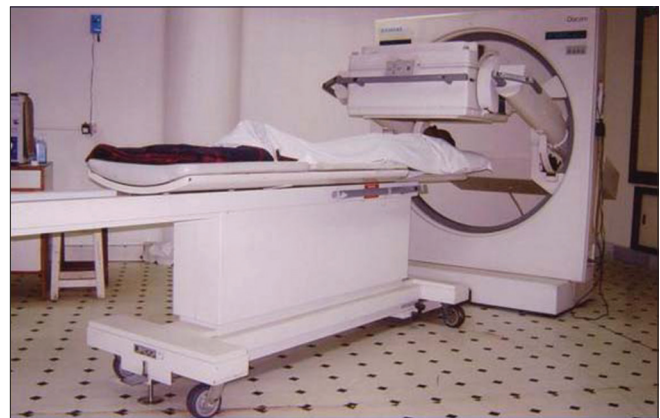
Figure 2: Gamma camera (siemens-diacam) with low energy all-purpose collimator
