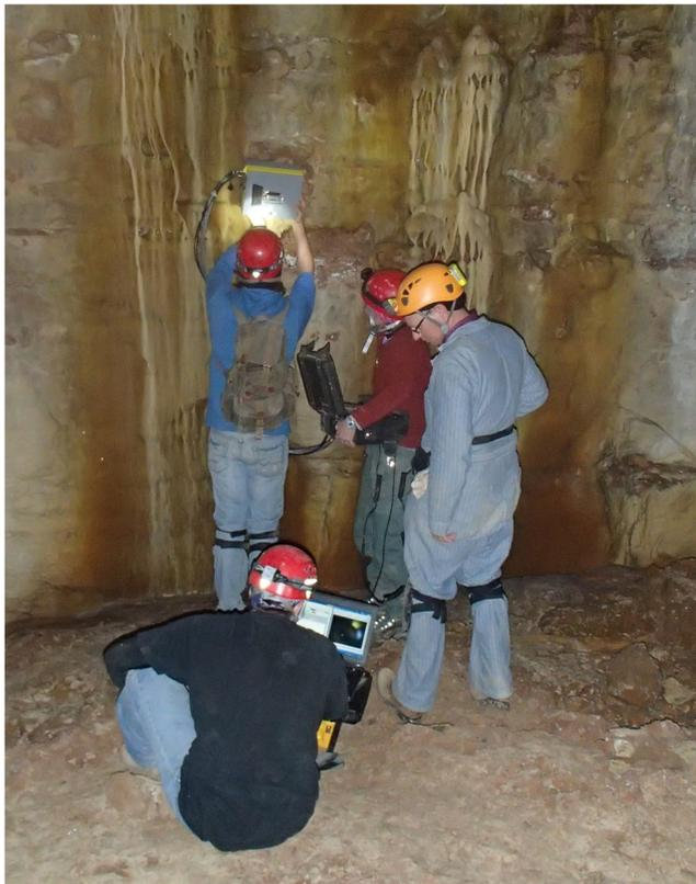
**Figure 7.** Data acquisition using portable acousto-optic spectrometer for astrobiology in Fort Stanton Cave on 31 October 2013. The acousto-optic tunable filter fixture is being held against a surface of interest while the data acquisition sequence is initiated on the laptop. The electronics module is tethered between the optics module and the laptop.
