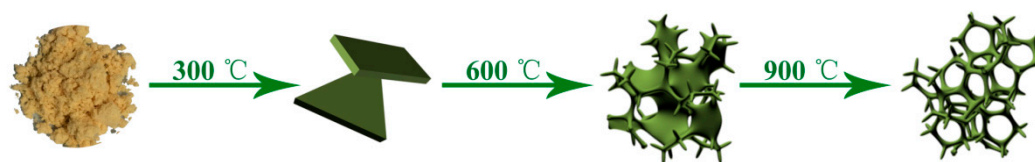
Scheme 1. Effect of temperature on the structure of obtained carbon materials.
