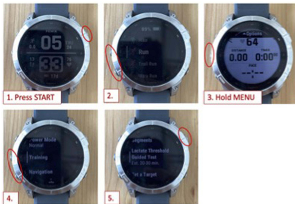
Figure 1 Procedure on Garmin watch face: getting to the guided lactate threshold test.
