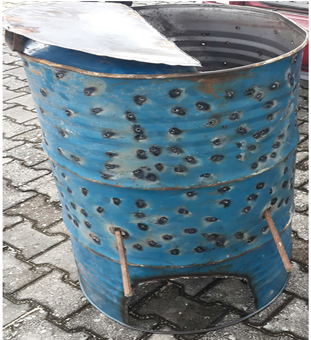
Fig 3. Field Incinerator. Locally made incinerator, improvised from a 220 litre drum based on WHO guidelines.
