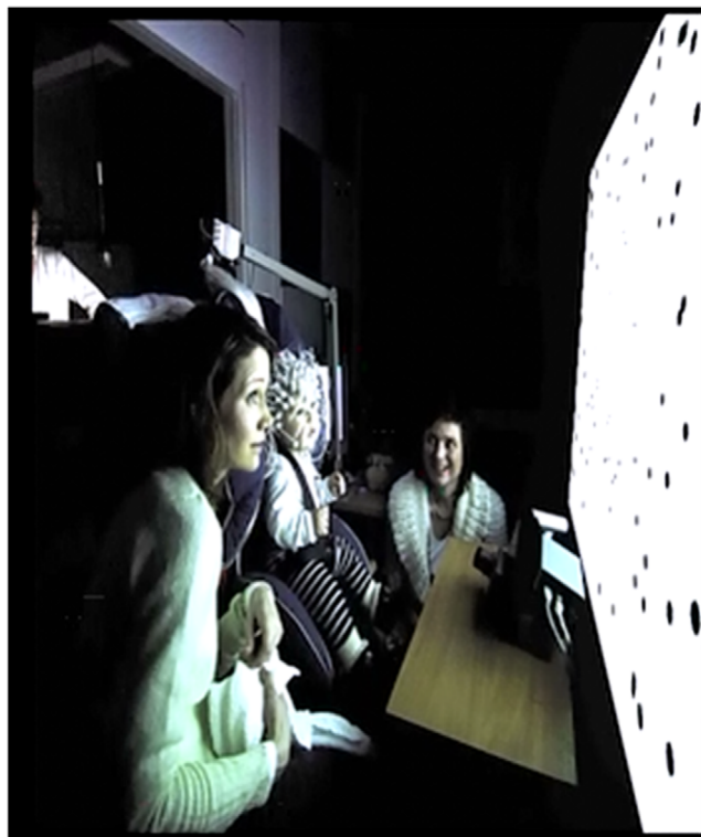
FIGURE 1 Showing the experimental set-up. Experimental room with a 9-month-old infant sitting in a baby car seat secured to an adjustable chair, wearing an electrode net consisting of 128 sensors. Moving dots simulating forward and reversed self-motion through optic flow and random visual motion, appeared on the large monitor in front of the infant (see also Video S1). The eye tracker was placed on the desk, between the participant and the screen, to monitor gaze. A parent and assistant were present during the entire session
