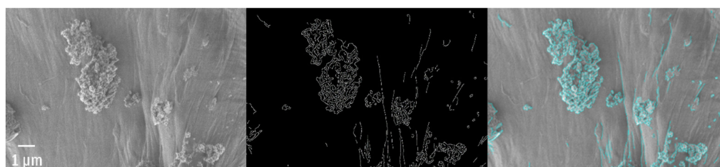
Figure 9. The rubbish bag with adsorbed material and the length of the total edge \sim 217.5 \mu\text{m} .
