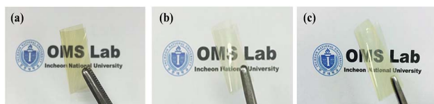
Fig. 1 Photographs of the crosslinked [xPI-PDMS-0.05][Br] (a), [xPI-PDMS-0.10][Br] (b) and [xPI-PDMS-0.15][Br] (c) membranes.
