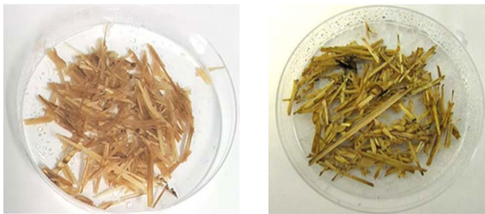
Figure 12. An example of visually notable fungus growth on untreated shredded straw that was submerged in water for 48 hours and then exposed to 21 days of fungal. (a) Untreated wood straw prior to (left), and 21 days after introduction of fungi (right).
