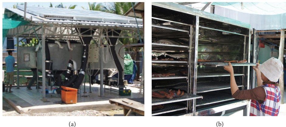
FIGURE 2: (a) Solar drying system (b) salted striped snakehead in solar drying chamber.
