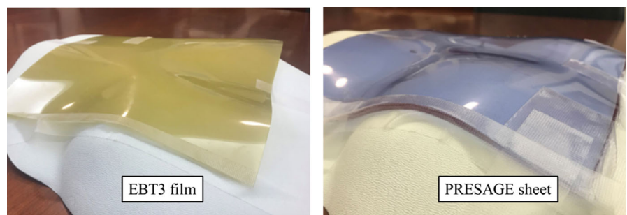
FIG. 2. EBT3 radiochromic film and PRESAGE sheet taped on a chest phantom. PRESAGE sheets conform better to irregular surfaces
