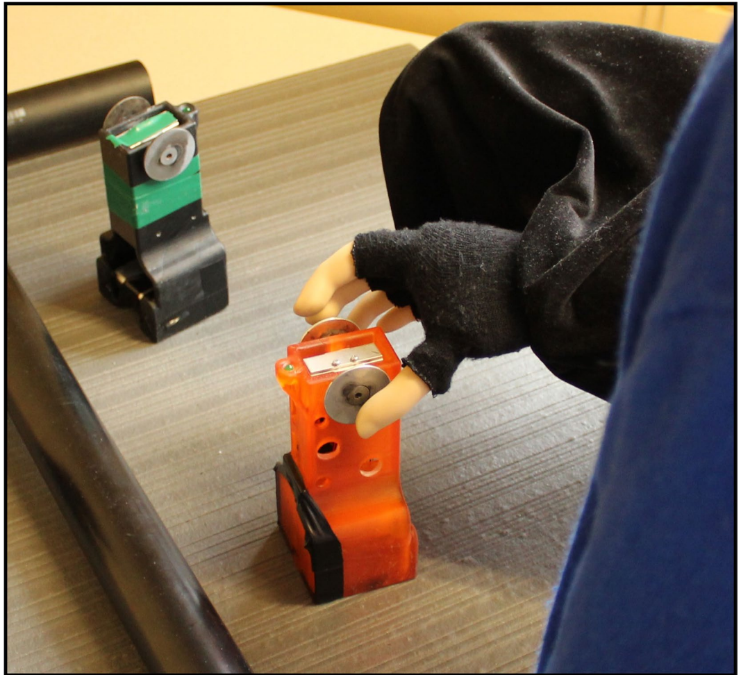
Figure 7. Variable weight mechanical eggs were moved during training periods. Load cells on eggs detected grasp force and simulated an egg breakage with a light cue when a threshold was exceeded.
