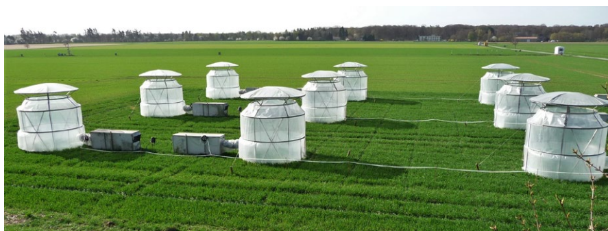
FIGURE 1 Part of the experimental field showing 9 out of the 12 open-top chambers
