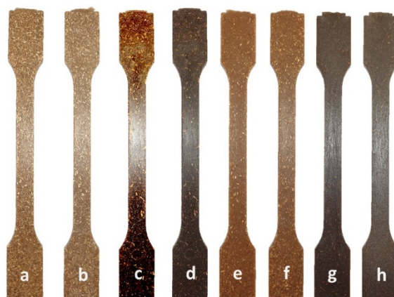
Figure 4. Test specimens of composites and biocomposites with halophyte biomass: (a) PP/Hemp20, (b) PP/Hemp30, (c) PP/Grass20, (d) PP/Grass30, (e) PLA/Hemp20, (f) PLA/Hemp30, (g) PLA/Grass20, (h) PLA/Grass30.
