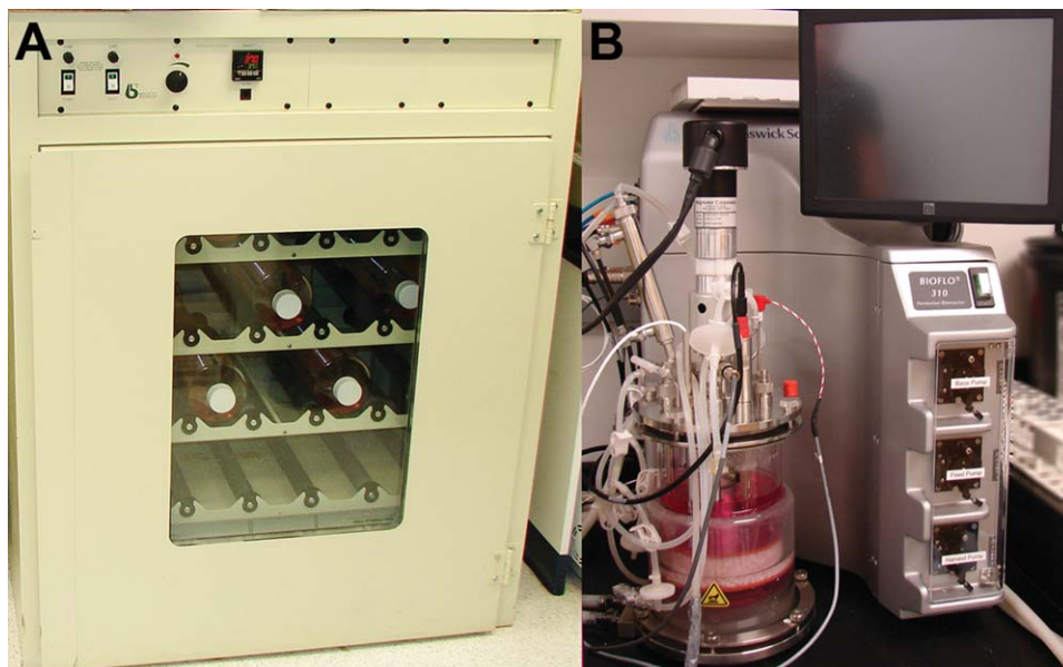
Figure 3. Large-scale growth of adherent 293H cell lines. (A) A mini 37°C roller incubator can hold up to 40 expanded surface pleated roller bottles at a time (equivalent to 10 L of media). (B) For larger volumes, 293H cells can be efficiently grown in a fiber cell packed-bed bioreactor similar to the BioFlo 310 for weeks to months at a time using either fed-batch or perfusion culture techniques.
