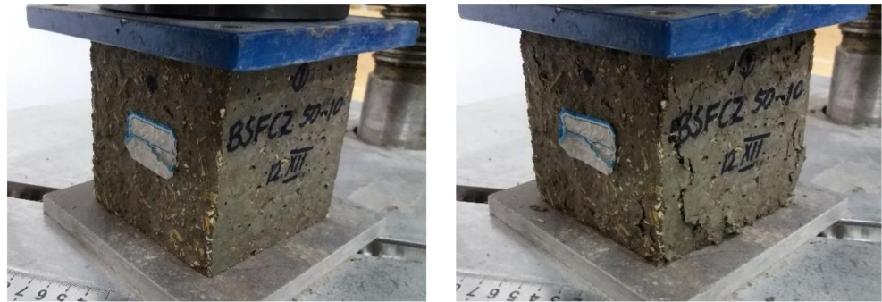
Figure 7. Composite specimen subjected to freeze-thaw cycles, before and after compressive strength testing.
