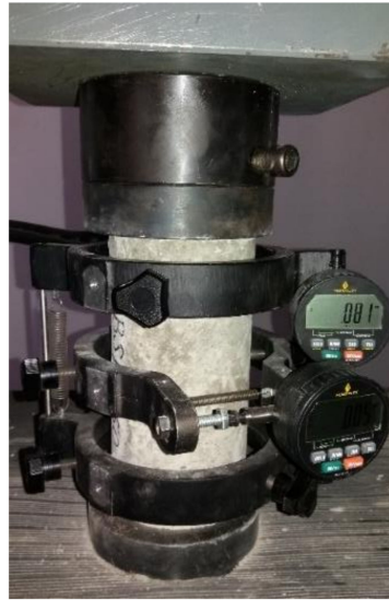
Figure 6. Modulus of elasticity testing.
