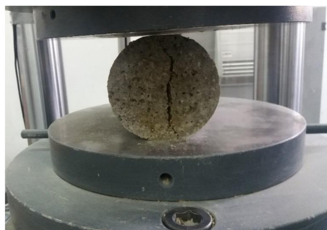
Figure 5. Splitting tensile testing.
