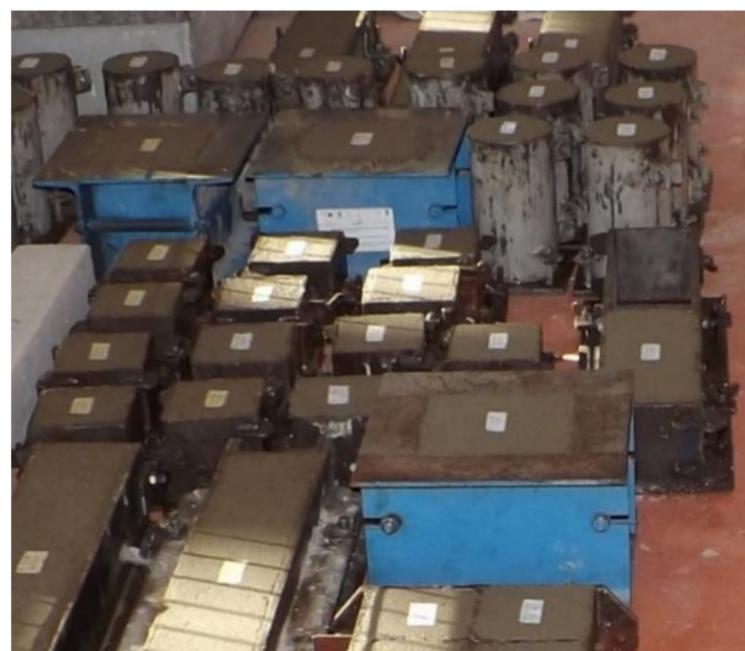
Figure 3. Composite specimens of a developed mix, in molds.
