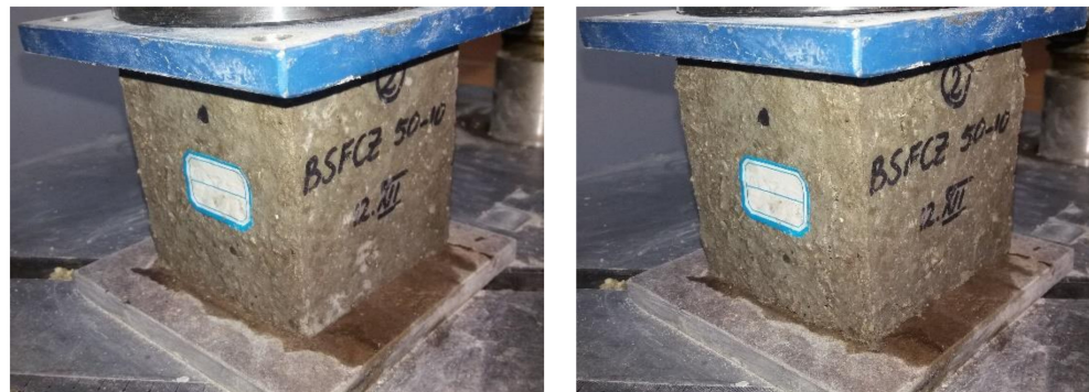
Figure 8. Composite control specimen, before and after compressive strength testing.
