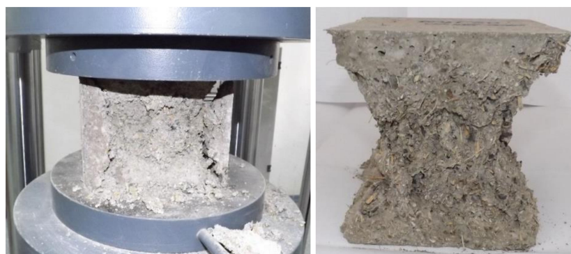
Figure 4. Compressive strength testing.
