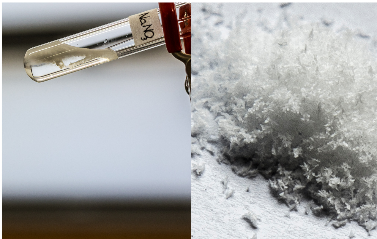
Fig 6. Nitrate salt of compound C1. Immediate precipitation after addition of C1 to aqueous NaNO 3 solution (left) and the recrystallized form (right).
