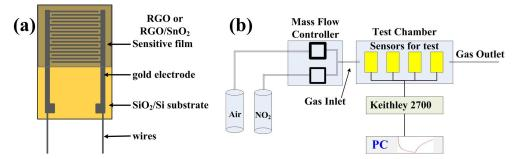
Figure 1. Schematic illustration of (a) the as-fabricated gas sensors and (b) measurement setup.
