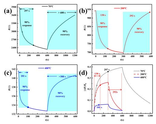
**Figure 7.** Response and recovery curves of sensors toward 50 ppm NO<sub>2</sub>. (**a**–**c**) Real-time resistance curves of sensors annealed at 70, 200, 400 °C, (**d**) real-time response curves.
