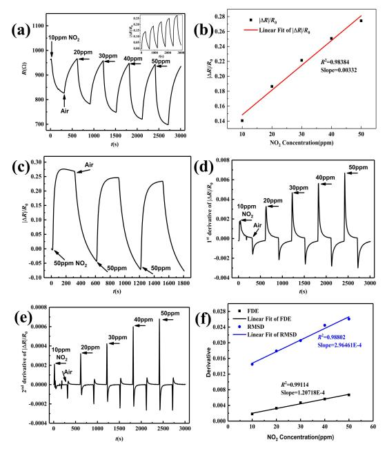
**Figure 8.** Sensing performance of 5.1%RGO/SnO<sub>2</sub> sensor (**a**) Real-time resistance change and response, (**b**) Sensitive, (**c**) Repeatability, (**d**) first derivative of response, (**e**) second derivative of response. (**f**) linear fit of FDE and RMSD.
