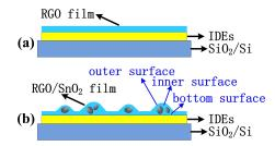
Figure 6. Schematic diagrams of (a) RGO film (b) RGO/SnO<sub>2</sub> composite film.
