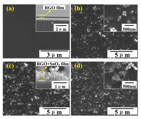
**Figure 2.** (**a**–**d**) SEM images of RGO, 9.7%RGO/SnO<sub>2</sub>, 5.1%RGO/SnO<sub>2</sub> and 2.6%RGO/SnO<sub>2</sub> film. The inset figures in (**a**,**c**) are cross-section images. The inset figures in (**b**,**d**) are magnification images.
