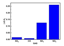
Figure 9. Selectivity of 5.1%RGO/SnO<sub>2</sub> sensor to 50 ppm SO<sub>2</sub>, CO, NH<sub>3</sub>, NO<sub>2</sub>.
