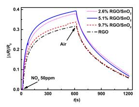
Figure 5. Responses of the sensors to 50 ppm NO<sub>2</sub> at room temperature.
