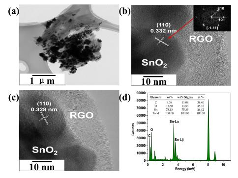
**Figure 3.** (a) TEM image, (b,c) HRTEM images and (d) EDX spectra of 5.1%RGO/SnO<sub>2</sub> nanocomposites. Inset in (b) presents the corresponding processed reduced FFT pattern of the HRTEM image.
