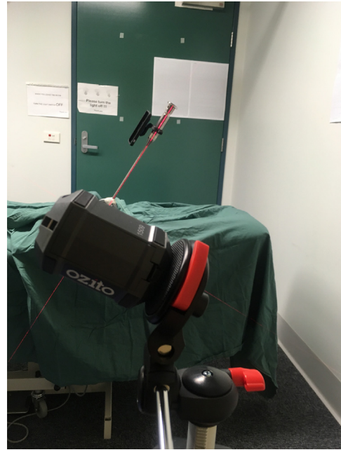
Figure 3. Laser beam aligned along the axis of the locked impactor and projected onto the sheets of graph papers in the background which were leveled to the “operating table” (using the SpiritLevel iPhone application).
