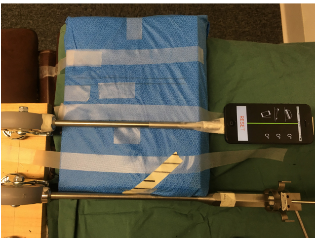
Figure 2. iPhone mounted on impactor (top) and Sputnik (alignment jig for 45 degree inclination and 15 degree anteversion) attached on impactor (bottom).
