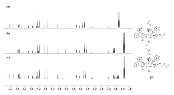
**Figure 8.** A comparison of the <sup>1</sup>H NMR (500 MHz, CDCl<sub>3</sub>, 298 K) spectra of the cyclic products (**a**) 6**a**, (**b**) 6**b** and (**c**) 6**c**. The singlet at  $\delta$  7.26 ppm in each spectrum is residual CHCl<sub>3</sub>. (**d**) The structures of 6**a** and 6**c** with atom labelling for NMR spectroscopic assignments (see Sections 4.5 and 4.6).
