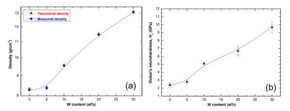
**Figure 9.** (a) Bulk density and (b) Vickers microhardness measure for SPS  $(Zr_{67}Cu_{33})_{100-x}W_x$  BMG consolidated system.
