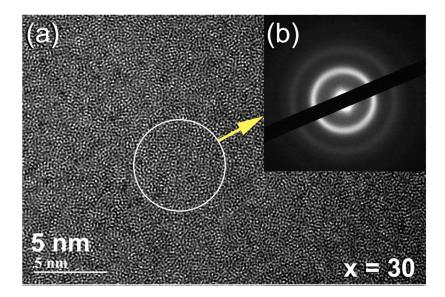
**Figure 4.** The FE-HRTEM micrograph and corresponding nano beam diffraction pattern (NBDP) of as-CR ( $Zr_{67}Cu_{33}$ )<sub>70</sub>W<sub>30</sub> for 100 passes and then BM for 75 h are displayed in (**a**) and (**b**), respectively.
