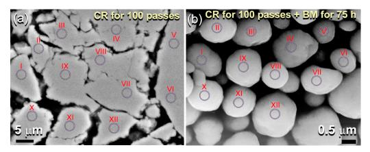
**Figure 3.** (a) FE-SEM micrographs of the cross-sectional view for ball milled  $(Zr_{70}Cu_{20}Ni_{10})_{80}W_{20}$  powders obtained after 12.5 h of mechanical alloying (MA) time. The high-magnification micrograph of the powders obtained after the final stage of MA (100 h) is displayed in (b) Zones.
