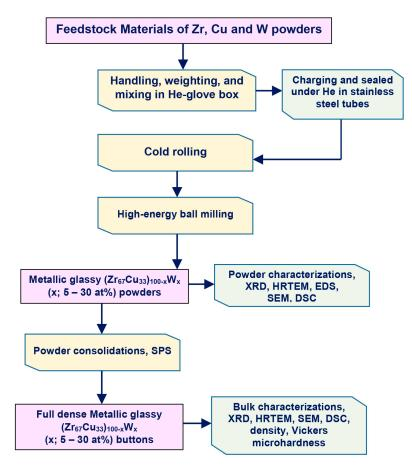
**Figure 10.** Flowsheet diagram presenting the experimental procedure followed in the present study for preparations and characterizations of metallic glassy  $(Zr_{67}Cu_{33})_{100-x}W_x$  materials.
