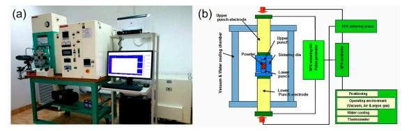
**Figure 11.** (a) A complete SPS system produced by Dr. Sinter Lab. Instrument, Japan housed in the Nanotechnology Laboratory, Energy and Building Research Center, Kuwait Institute for Scientific Research, and (b) schematic illustration of the system configuration.
