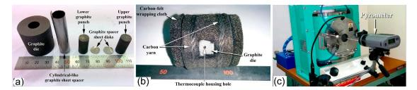
**Figure 12.** (a) Powder loading kits used in SPS consisting of graphite die and punches, cylindrical graphite spacer and graphite disk spacer, (b) the die containing the powder was wrapped by carbon-felt and tight with using carbon yarn, and (c) the surface temperature of the die was monitored during the SPS process, using a pyrometer.
