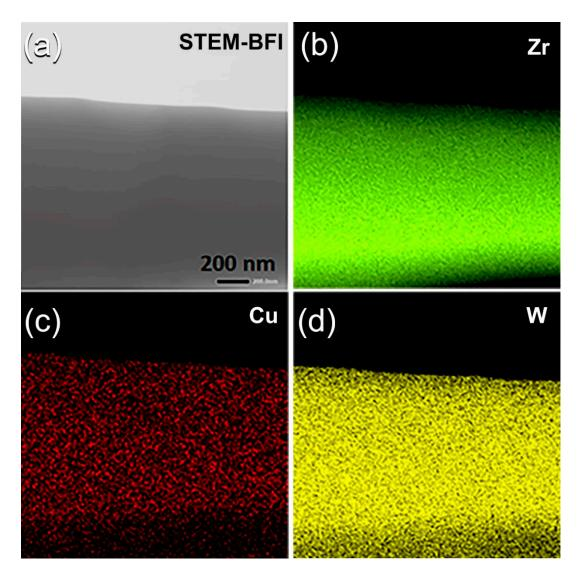
**Figure 8.** (a) Scanning transmission electron microscope-bright field image (STEM-BFI) and corresponding X-ray EDS elemental mapping of (b) Zr, (c) Cu, and (d) W for a sliced  $(Zr_{67}Cu_{33})_{70}W_{30}$  BMG sample.
