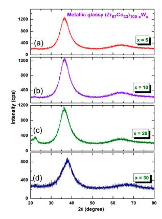
**Figure 5.** XRD patterns of  $(Zr_{67}Cu_{33})_{100-x}W_x$  powders with *x* equals to (**a**) 5, (**b**) 10, (**c**) 20, and (**d**) 30 at%. The samples were obtained after CR for 100 passes followed by 75 h of BM.
