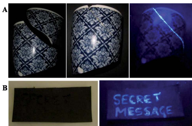
Fig. 9 (A) The picture depicting the bonding of a broken specimen design (left) by P(VP-Acn-Acr) and the visibility of the broken joint under normal light (middle) and long-wavelength UV light (right); (B) the figure depicting the visibility of the words written by the adhesive under UV light (365 nm), which are invisible under normal light.
