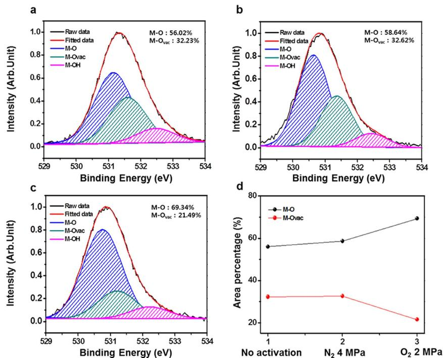
**Figure 5.** The O 1s peaks of XPS analysis in a-IGZO channel layer under different conditions (a) no activation, (b) N<sub>2</sub> 4 MPa at 100 °C, and (c) O<sub>2</sub> 2 MPa at 100 °C. (d) Area ratio of M-O and M-O<sub>vac</sub> in each condition.
