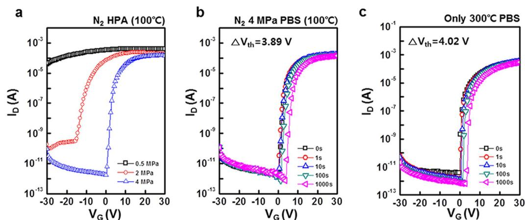
**Figure 2.** (a) Transfer characteristics of HPA activated a-IGZO TFTs varying  $N_2$  pressure at  $100^\circ\text{C}$ , and PBS test results of HPA activated a-IGZO TFTs under (b)  $N_2$  4 MPa at  $100^\circ\text{C}$  (c)  $300^\circ\text{C}$  for 1000 s.
