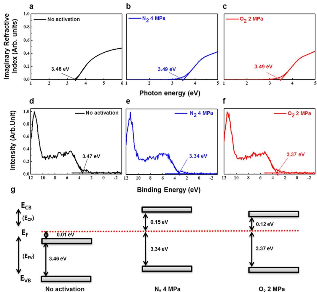
**Figure 6.** (a–c) Imaginary part of SE spectra absorption coefficient, (d–f) XPS spectra near the valence band and (g) band alignment of a-IGZO channel layer under different conditions: no activation,  $O_2$  2 MPa at 100 °C, and  $N_2$  4 MPa at 100 °C.
