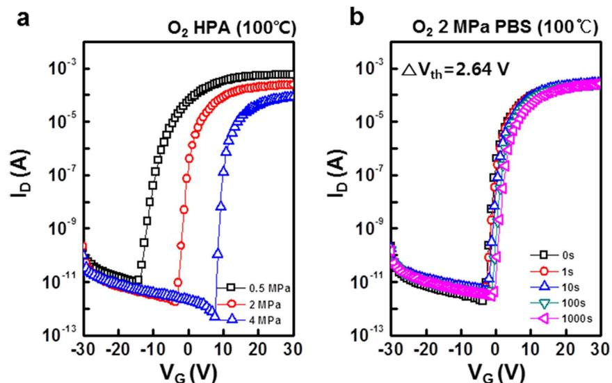
**Figure 3.** (a) Transfer characteristics of HPA activated a-IGZO TFTs varying  $O_2$  pressure at  $100^\circ C$  (b) PBS test result of HPA activated a-IGZO TFTs under  $O_2$  2 MPa at  $100^\circ C$ .
