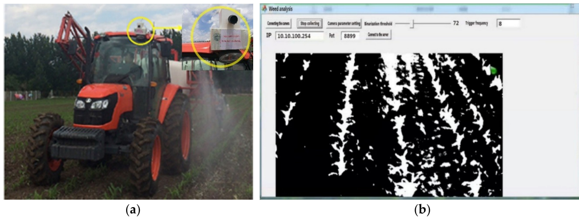
Figure 1. Imaging system used in study: (a) The variable-rate sprayer integrated imaging sensor (in yellow circle) for weed detection; (b) The imaging system interface.
