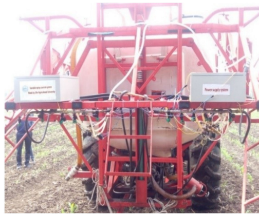
Figure 6. Field testing of the variable-rate spraying system.
