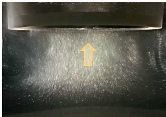
Fig. 8. Visualization of the current lines generated by stirring.
