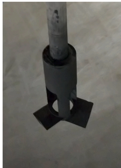
Fig. 4. Graphite blade connected to alumina hollow rod.
