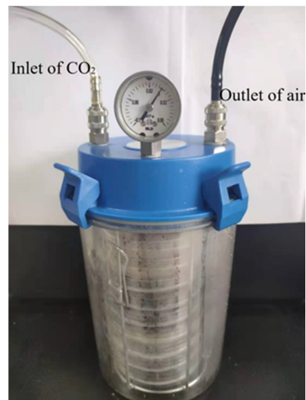
Figure 2. Instruction of anaerobic jar.
