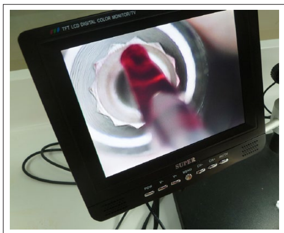
Figure 2. Placement of Rhodamine B solution inside the implant.
