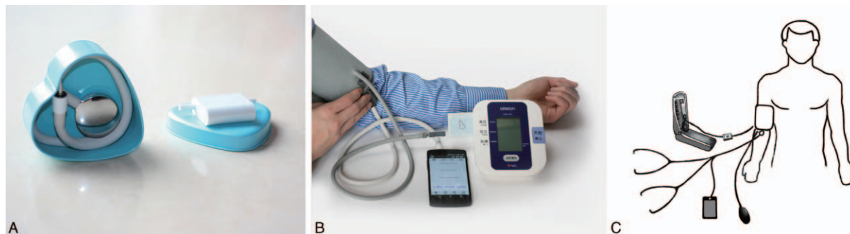
Figure 1. Monitor photograph: The main components of the Accutension are shown in (A). The component in the left is auscultation head equipped with a microphone which collects Korotkoff sounds and transfers them to the smartphone. The component in the right is pressure sensing and Bluetooth communication module. (B) By seamlessly accessing to the Omron oscillometric BP monitor, Accutension can acquire a second reading simultaneously from it. (C) Accutension works with mercury sphygmomanometer by incorporating into it. Two observers and Accutension share 1 stethoscope head by 2 Y-tube connectors.
