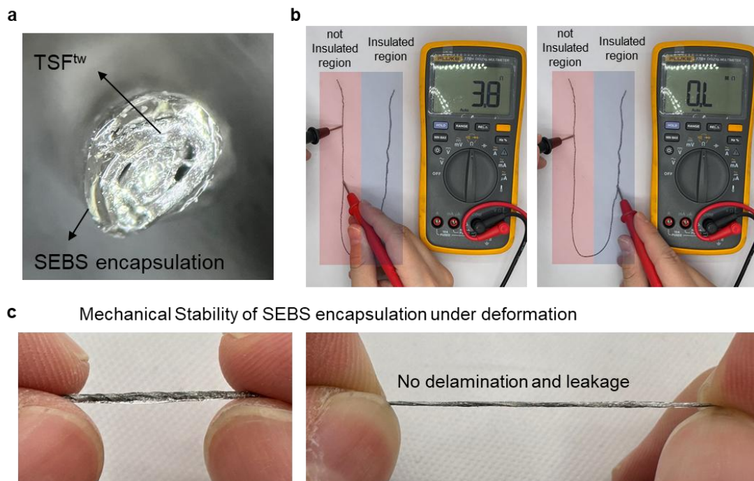
Supplementary Fig. 33| SEBS coating on TSF tw . a , Cross-sectional OM image for SEBS-coated TSF tw . b , Photograph of TSF tw without and with SEBS coating. c , Photograph of stretched SEBS-coated TSF tw .
