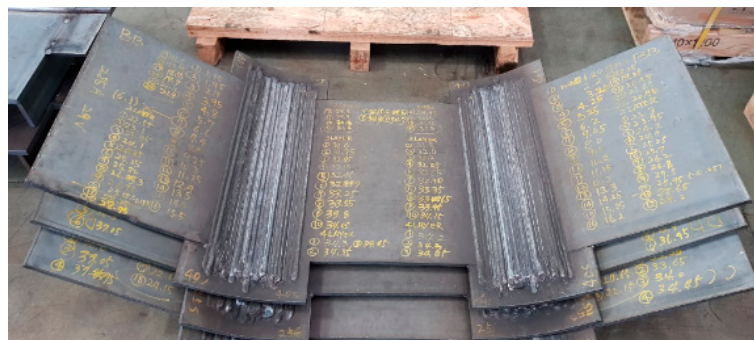
Figure 3. Welded specimens used to measure angular distortion.
